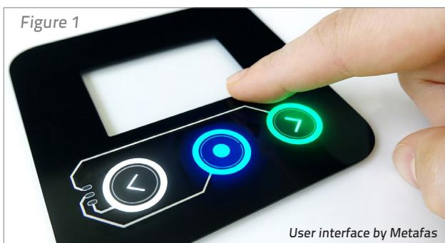
respond to the touch actuation. The product is made by a combination of screen-printed PEDOT touch electrodes and inkjet printed silver traces. The transparency of PEDOT electrodes allows for the backlighting and lightguide. Figure 2 shows this transparency of the blueish PEDOT electrodes printed on a PEN film.
