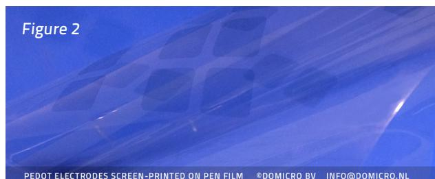
PEDOT ELECTRODES SCREEN-PRINTED ON PEN FILM ©DOMICRO BV INFO@DOMICRO.NL
