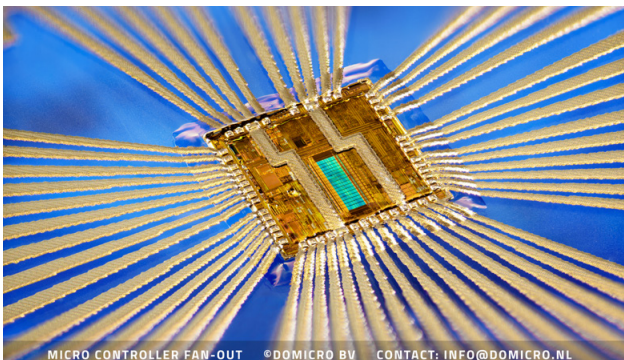
Figure 1. Inkjet printed wire bonds for the interconnection of microprocessor bare die
